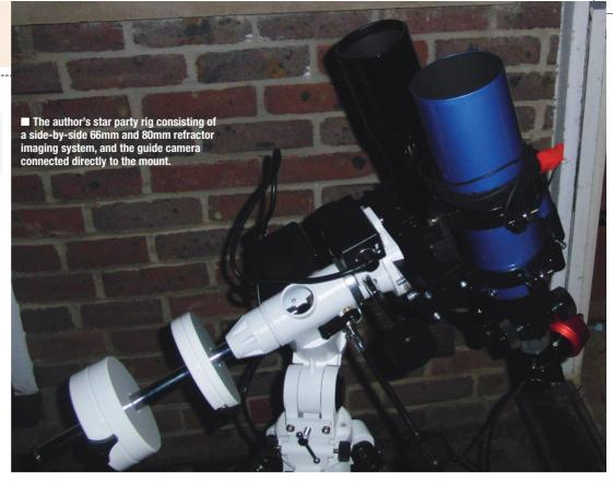
out of the observatory with one hand. If you treat the weight limits with respect (and in my set-up's case, it's about four kilograms in total), then this tiny set-up, which can break down to fit easily into a suitcase for travelling (eclipses and special events), has the potential to revolutionise the portable astronomy market. Whilst other products exist for the travelling astronomer, this one seems to have it all.
